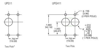
Panel Mounting Detail: Tolerance ±.005 [.13] unless noted.
