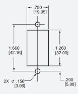
Panel Mounting Detail: Tolerance ±.005 [.13] unless noted.
